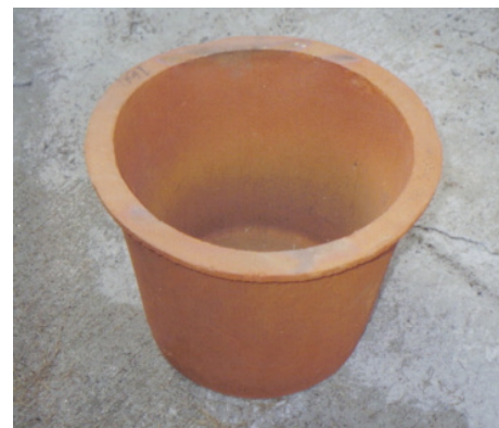
The Potters for Peace filter, locally produced in Nicaragua (CDC / D. Lantagne)
